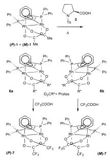
placement of acetate by Protos in the orthometalated acetate mixture (P)-1 and (M)-1 yielded the expected 1:1 mixture of the desired diastereomers 6a and 6b. These were separable by silica gel chromatography.9
